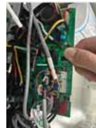
6. Pull out the PCB and unplug the refrigerant leak sensor from CN3.
