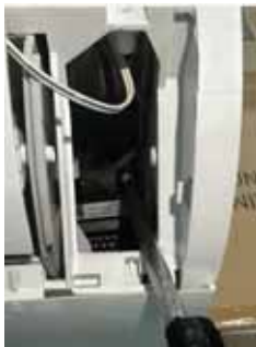
3. Remove leak sensor.
