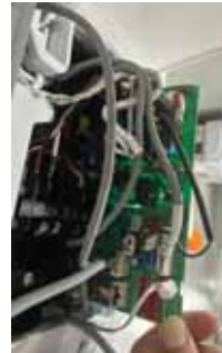
4. Pull out the PCB and unplug the refrigerant leak sensor from CN3.
