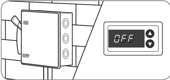
**At initial start-up or after extended shutdown periods, make sure the crankcase heater is energized for at least 12 hours before the compressor is started. (Disconnect switch is on and wall thermostat is off.)**
