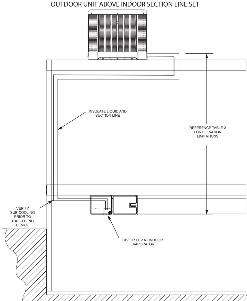
For applications that are considered to have a long line set with the outdoor unit above the indoor unit the following is required:
