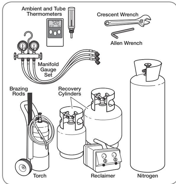
**Pressure:** The pressure of R-410A is approximately 60% (1.6 times) greater than R-22. Recovery and recycle equipment, pumps, hoses, and the like must have design pressure ratings appropriate for R-410A. *Manifold sets need to range up to 800 psig high-side and 250 psig low-side with a 550 psig low-side retard. Hoses need to have a service pressure rating of 800 psig. Recovery cylinders need to have a 400 psig service pressure rating, DOT 4BA400 or DOT BW400.*
