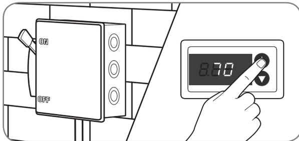
With thermostat in the “Off” position, turn on the power to the furnace or air handler and the condensing unit. Start the condensing unit and the furnace or air handler with the thermostat. Verify that the outdoor unit is operating and the indoor air mover is delivering the correct airflow for the system size.
