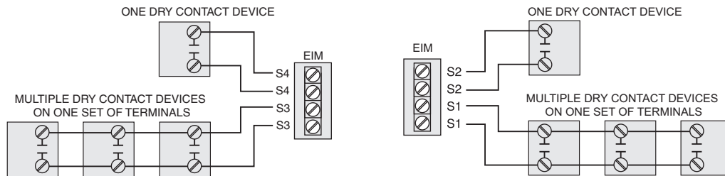
Fig. 157. Wiring dry contact devices.
