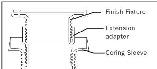
Install adapter into female threads of Coring Sleeve. Install Finish Fixture into female threads of adapter. Adjust to proper height. Apply silicone adhesive to threads if desired.
