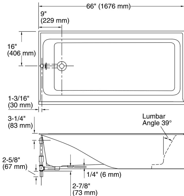
No change in measurement if connected with drain illustrated. (K-7259)
