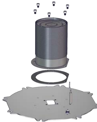
Figure 63 Removing bolts securing burner to heat exchanger lid
