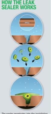
The sealer penetrates into the installation with micro-leaks, binds, polymerizes and seals the leakage points.
