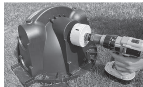
2. Drill the hole on the endcap.
