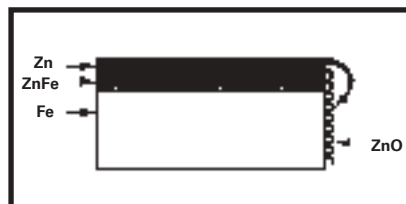
Protection of cut edges with zinc coatings.
