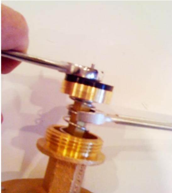
2. Remove seat disc, disc holder and spring from the shaft.
