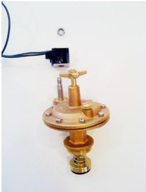
2. Using a flathead screwdriver, unscrew and remove solenoid post from top of adaptor.
