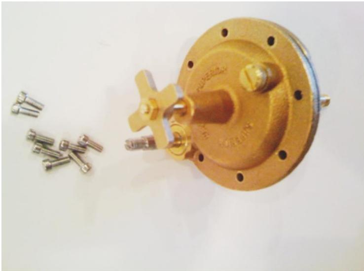
4. Lift top straight up until metering rod clears the top of the diaphragm shaft. It may be necessary to pry the top loose from lower housing using a flathead screwdriver.
