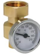
Point of distribution mixed temperature gauge adaptor fits MixCal 521 series mixing valves. Threaded union mounting replaces existing mixed outlet with 3/4" or 1" sweat pipe connection. Removable gauge fits into temperature well. Gauge dial is 2" diameter and scale from 30–210° F. Low-lead brass body.
