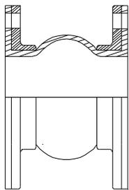
**Global-Flex Mfg. Style REJM** expansion joints are the ultimate in quality molded construction. Premium grade elastomers provide long service life in the most demanding applications. For superior performance and pressure ratings, Global-Flex **Style REJM** expansion joints have a minimum *4 to 1* safety factor built in to their rated operating pressures. Working pressure up to 200 psi.
