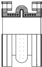
**Global-Flex Mfg. Style REJ-TN** expansion joints combined the best features of Teflon with the best features of elastomeric expansion joints. Joints are available in 1” up to 24” I.D. in standard face-to-face dimensions, or special lengths. Also available in multiple arch configurations or as straight pipe.
