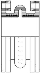
**Global-Flex Mfg. Style REJZ** expansion joints are the ultimate for use in low spring rate applications. The light weight construction lowers forces exerted on the mating flanges. This improved flexibility allows for easier installation.
