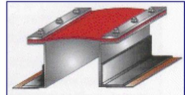
A single layer belt with chemical barrier is suggested in either integrally flanged or flat belt type. Such as the weld-in outboard angle frame design and Teflon® coated single layer belt with gas film shown.
