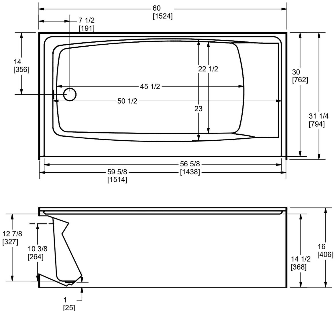
Measurement tolerances  $\pm 1/4"$  (6.3mm)
