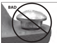
OVAL NECK OF BOLT NOT SEATED PROPERLY
