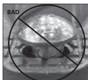
OVAL NECK OF BOLT NOT SEATED PROPERLY
