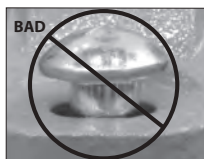
OVAL NECK OF BOLT NOT SEATED PROPERLY
