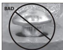
OVAL NECK OF BOLT NOT SEATED PROPERLY
