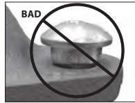
OVAL NECK OF BOLT NOT SEATED PROPERLY
