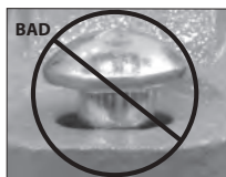
OVAL NECK OF BOLT NOT SEATED PROPERLY
