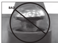
OVAL NECK OF BOLT NOT SEATED PROPERLY
