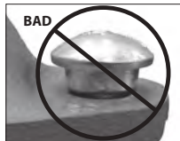
OVAL NECK OF BOLT NOT SEATED PROPERLY
