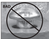
OVAL NECK OF BOLT NOT SEATED PROPERLY
