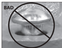
OVAL NECK OF BOLT NOT SEATED PROPERLY
