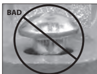
OVAL NECK OF BOLT NOT SEATED PROPERLY
