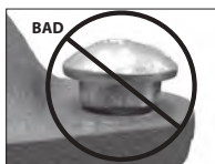
OVAL NECK OF BOLT NOT SEATED PROPERLY
