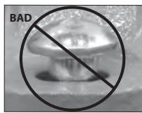
OVAL NECK OF BOLT NOT SEATED PROPERLY
