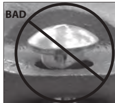
OVAL NECK OF BOLT NOT SEATED PROPERLY
