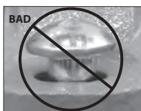
OVAL NECK OF BOLT NOT SEATED PROPERLY
