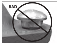
OVAL NECK OF BOLT NOT SEATED PROPERLY
