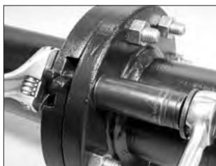
4-Bolt Tightening Pattern
