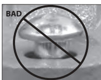
OVAL NECK OF BOLT NOT SEATED PROPERLY
