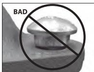
OVAL NECK OF BOLT NOT SEATED PROPERLY
