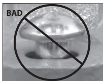
OVAL NECK OF BOLT NOT SEATED PROPERLY
