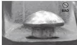
BAD BOLT ENGAGEMENT (OVAL NECK OF BOLT IS NOT SEATED PROPERLY IN THE BOLT HOLE)
