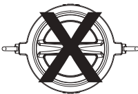
Incorrect Orientation for Horizontal Installation
