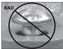
OVAL NECK OF BOLT NOT SEATED PROPERLY
