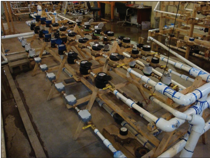
This gravimetric test bench was used to analyze mechanical and electronic meter accuracy for this study at the Utah Water Research Laboratory in Logan, Utah. Photo courtesy of Utah Water Research Laboratory.
