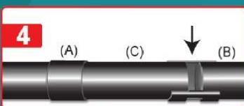
Using 1/2 of Exact Fit coupling
