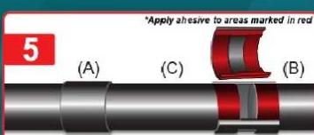
Apply adhesive to pipes B&C and
