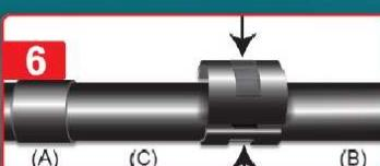
Install both halves of Snap-Lock
