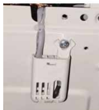
Ambient Temperature Sensor
