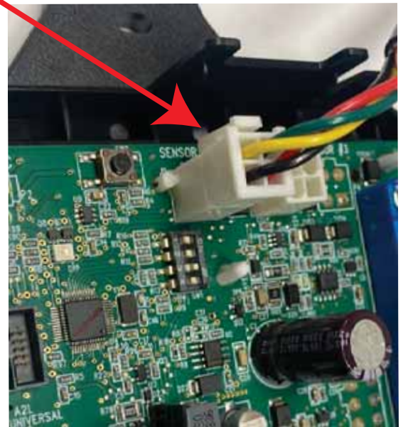
Figure 4. Connecting the RDS Sensor to RDS Non-Communicating Blower Control Board
