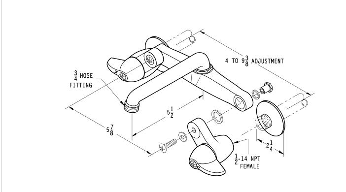
Ø1-3/8 Min to Ø1-1/2 Max. Deck Hole Opening
