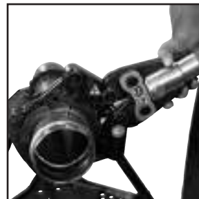
Figure 8: Placement of adapter jaw into pressing chain
