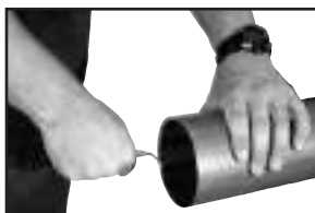
Figure 3: Deburr inside diameter deburring tool
