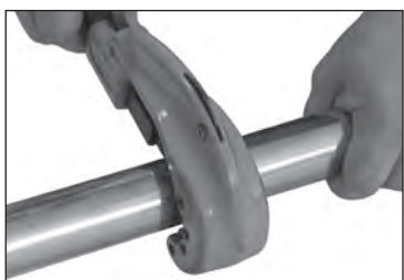
Figure 1 — Cut tube to desired length
