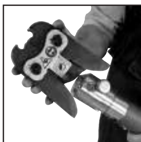
Figure 7: Placement of adapter jaw into the tool
