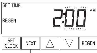
STEP 5I – Next Regeneration Time (minutes): Set the minutes of day for regeneration using ▲ or ▼. This display will not be shown if “on 0” is selected in Step 10S or Step 8F. Press NEXT to exit Installer Display Settings. Press REGEN to return to previous step.
