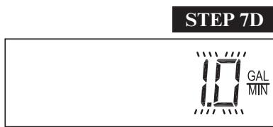
**STEP 7D** – Flow rate, maximum last seven days: The maximum flow rate in gallons per minute that occurred in the last seven days will be displayed. This display will equal zero if a water meter is not installed. Press and hold **▲** and **▼** for approximately 3 seconds to reset to zero. Press **NEXT** to go to Step 8D. Press **REGEN** to return to previous step.
