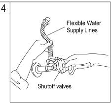
4. Connect the water supply lines. Before connecting the supply lines, apply pipe joint compound to the threads on the inlet shanks and shut off valves.
