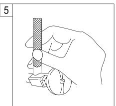
5. Turn on water supply valves and check for leaks, especially at hook-ups to supply
