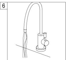
6. Turn On your filtration faucet and allow water to run for one minutes to make sure installation set up completed. Note: Aerator is attached to spout and not
