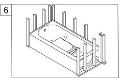
6. Secure to the wall with galvanized screws at the predrilled screw location, apply weight to the middle of the tub until the mortar sets.
