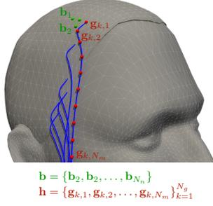
**Figure 2: Hair and body parametrization:** We represent hair using control points on a sparse set of guides and body using vertices making up the triangular mesh of bust.
