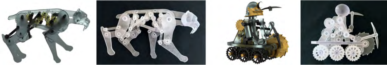
Figure 1: The interactive design system we introduce allows non-expert users to create complex, animated mechanical characters.
