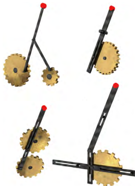
Figure 4: We assume as input a library of parameterized driving mechanisms such as the ones illustrated here. These building blocks are instantiated by our framework, optimized and attached to the input character, driving its motion. The locations of the attachment points are highlighted.
