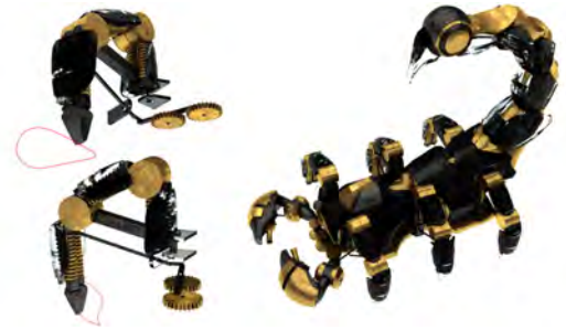
Figure 15: Scorpio character, showing 3D motion. Left: Leg and driving mechanism in isolation. Right: Simulated character walking.
