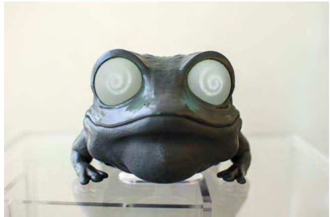
Figure 1. Curved displays are embedded into the character to design interactive eyes. The character itself is passive and does not have any electronics embedded.
