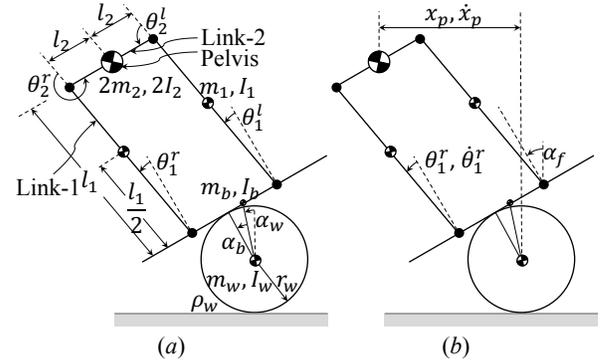
Fig. 2: Bongoboard dynamic model: (a) With its configurations and system parameters marked; and (b) With its five outputs used for output feedback control marked.
