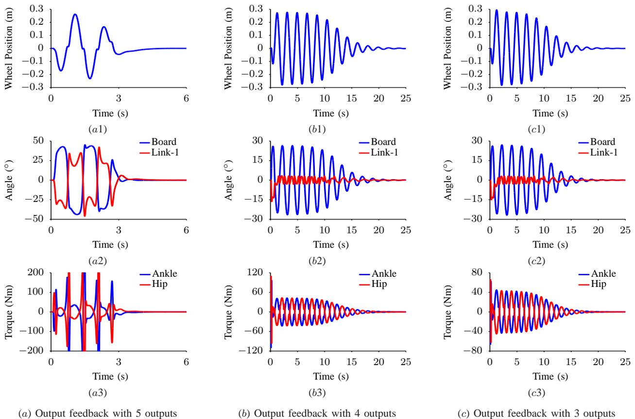
Fig. 5: Output feedback controllers' successful efforts in stabilizing bongoboard models when subjected to the following board disturbances for 0.1 s: (a) 87.2 Nm, (b) 57.4 Nm, and (c) 54.5 Nm.
