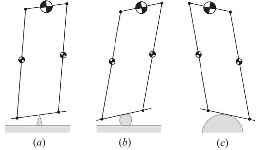
Fig. 1: Balancing in different dynamic, unstable environments: (a) Seesaw, (b) Bongoboard, and (c) Board on a curved floor.
