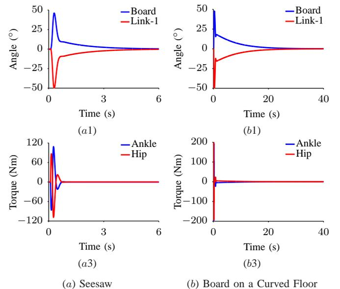
Fig. 4: Output feedback controllers' successful efforts in stabilizing seesaw and curved floor models with three outputs when subjected to the following disturbances for 0.1 s: (a) 60.7 Nm, and (b) 194.8 Nm.
