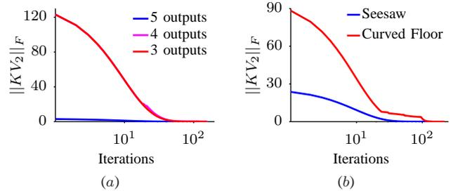
Fig. 3: Semi-logarithmic plots of the Frobenius norm  $\|KV_2\|_F$  converging to zero producing stabilizing output feedback controllers using Algorithm 1: (a) Bongoboard model with different number of outputs, and (b) Seesaw and curved floor models with three outputs.
