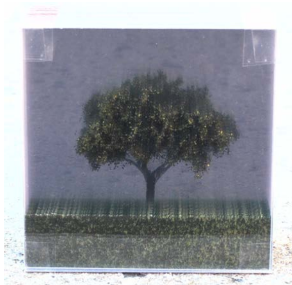
Figure 14: A 10-layer model of a tree constructed from polycarbonate and acetate sheets, viewed from approximately 20^\circ above the principal view direction. Objects with very thin features such as this tree cannot be printed using additive 3D printers.
