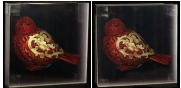
Figure 11: Left: A multilayer model printed using polycarbonate and acetate sheets without accounting for attenuation and multiple scattering. Right: The same model printed after applying these corrections. This model is composed of seven layers of polycarbonate with acetate sheets. Note how the brightness and contrast of the front-most layers match the back layers in the corrected model.
