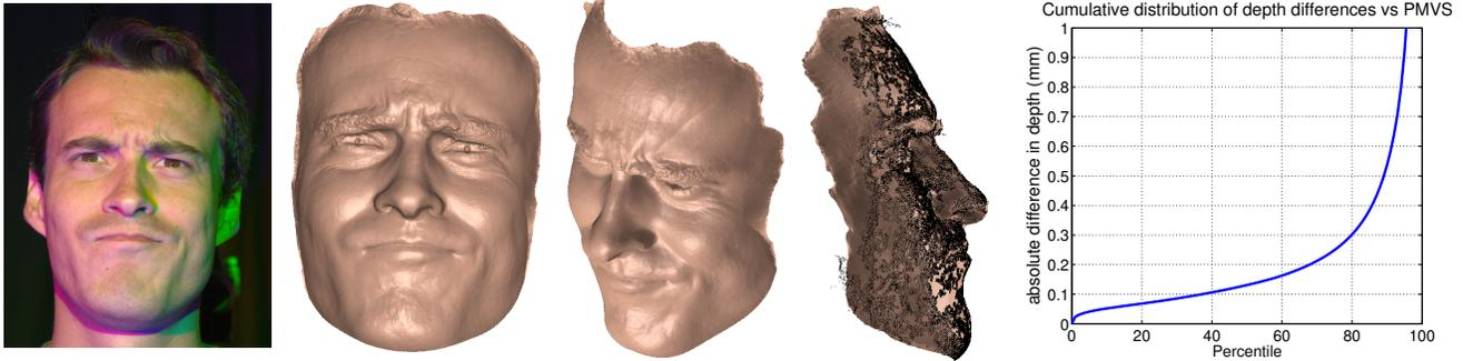
Figure 2. Detailed 3D reconstruction for a real frame in the supplementary video. The face profile view is overlaid with the PMVS point cloud, showing close agreement in recovered depth (median difference of 0.13 mm, 90<sup>th</sup> percentile at 0.5 mm, over 100 frames).
