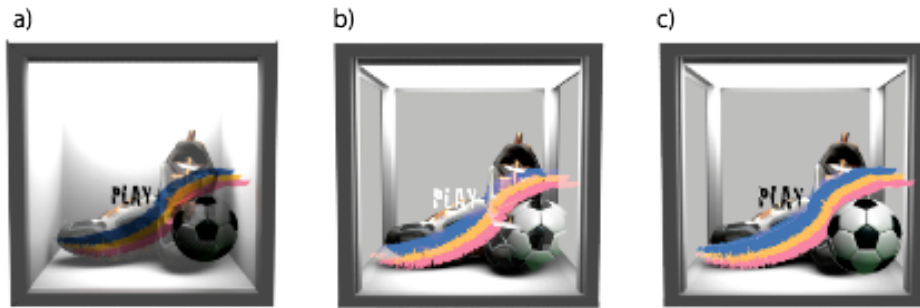
Figure 1a,b,c. Transparent Displays. a) absorbing (e.g.LCD) b) emissive (e.g.OLED) c) ideal absorbing and emissive.
