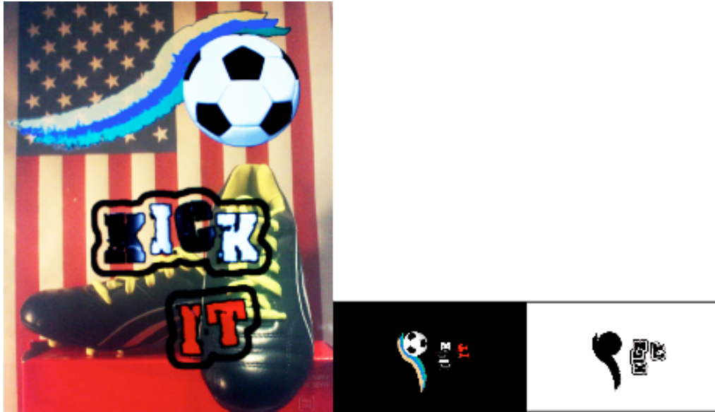
Figure 7a,b,c. a) Opaque emissive content on transparent field from prototype display. Corresponding b) content and c) mask image frames.
