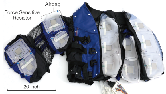
Figure 3. Force Jacket with internal airbags layout exposed.
