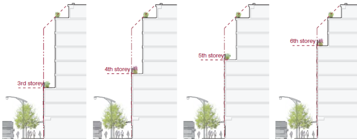
For buildings taller than 23 metres, an additional step-back may be required. The location of this step-back is flexible. The above example illustrates a 9 storey building on a 30 metre R.O.W. which integrates step-backs in accordance with Performance Standard 4A: Front Façade: Angular Plan and an additional Pedestrian Perception step-back.
