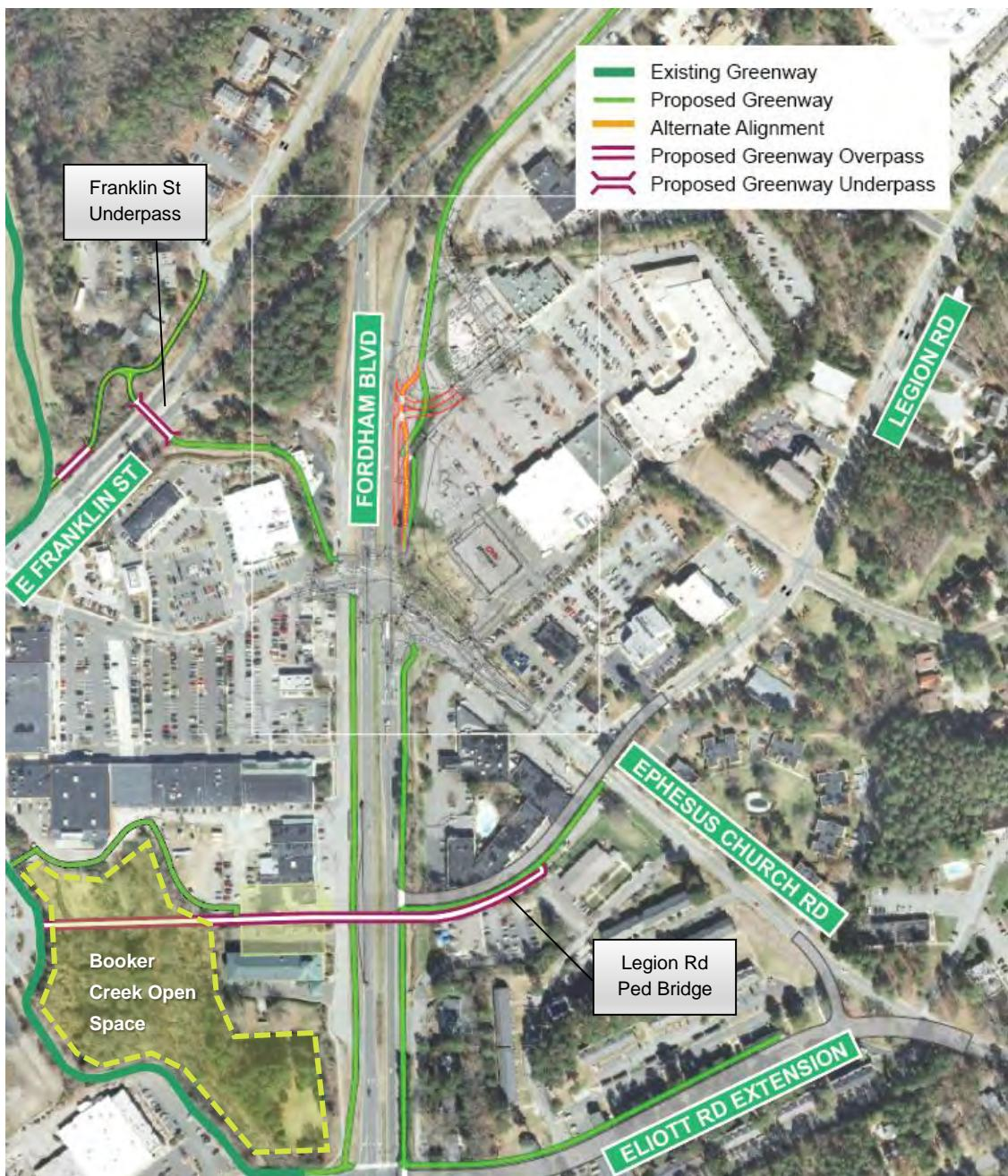
**Figure 10.** Recommended multi-use bridge concept across Fordham Boulevard at Legion Road Extension, with extension over Booker Creek open space, including the design perspective below
