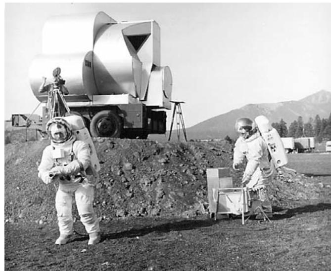
Field testing at Cinder Lake Crater. Flagstaff USGS geologists, acting as astronauts, tested the simulated Lunar Module for future training exercises.
