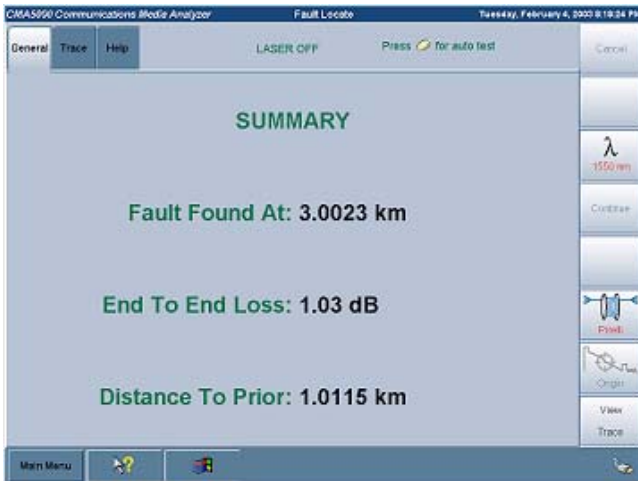
Fig.1: Fault Locate Mode - ease to read results
