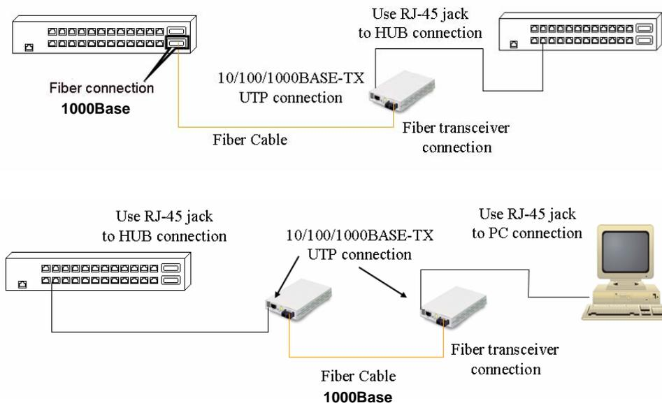
The following example illustrates the connection scheme when connecting from a 1000BASE-TX port of one HUB to a 1000BASE-TX Network Interface Card (NIC) in a computer through the fiber converter.
