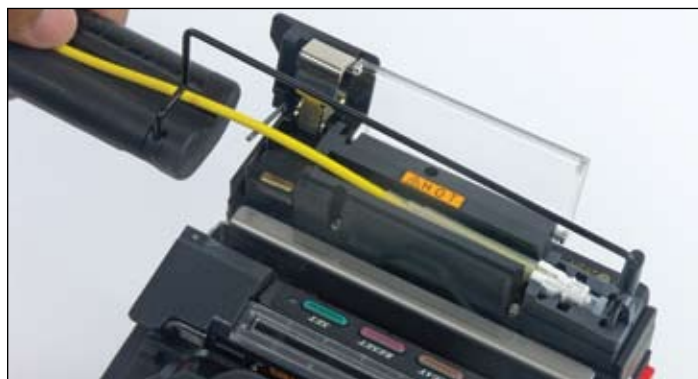
FIGURE 8 — Inserting Connector Body into Tube Heater
