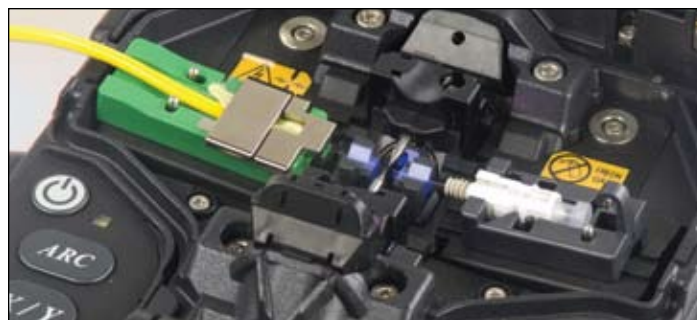
FIGURE 6 — Placing Fiber Holder & Connector into Splicer
