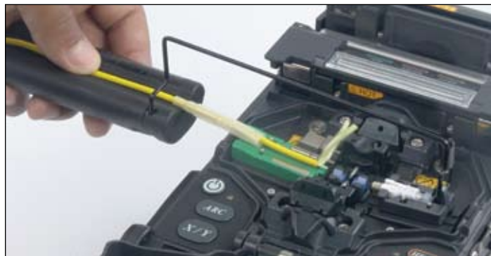
FIGURE 7 — Insert Transfer Tool into Connector Body Holder
