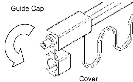
2. Insert tip of cleaner into LC Adapter
