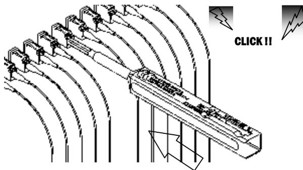
Be careful not to slant the IBC Brand Cleaner LC while inserting into the adapter.
