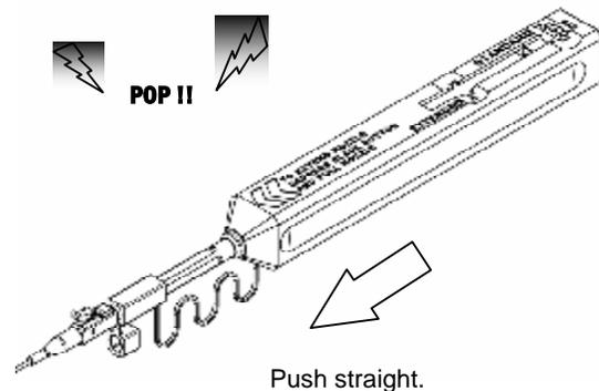
Be careful not to slant LC connector while inserting into the Guide cap.
