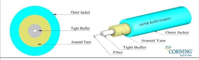
The Light Connections Simplex Cable is composed of a tight buffer, aramid yarn, and a PVC outer jacket. All component materials meet the EU RoHS and REACH Directive standards.
