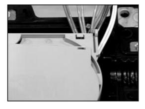
4.03 Lay the buffer tube ends over the channels. If tubes are too long to fit in channels, trim excess off. DO NOT CUT FIBERS.
