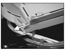
6.02 Now slide the tray laterally (flexing the lever arm outward) enough to allow the post to be inserted into the opposite lever arm hole. (Back view shown).
