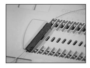
5.05 Prior to placing the splice into the pocket, observe how the splice lays in its relaxed state. Rotate the splice through the smallest possible angle. Snap splice into pocket cap side down.
