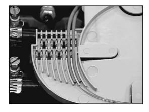
4.05 Lay at least one complete loop of fiber from the first buffer tube on the tray with the fiber ends crossing the <u>front</u> "CUT HERE" mark.
