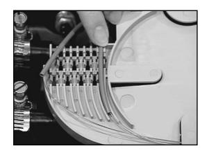
4.04 Press the buffer tube into the channel to secure. The buffer tube should stop within 1/4" (6 mm) of the channel end.
