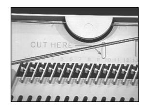
4.10 Now cut the fiber ends at the mark. Be sure to cut <u>ONLY</u> the fiber ends.
