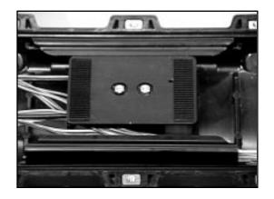
3.12 Cut the Dual-Lok to fit the four flat pads on the tray bottom. Remove protective liner and adhere.
