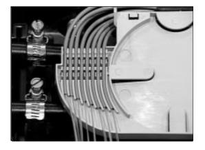
5.02 Remove the minimum length of fiber required to prepare and splice the fibers.
