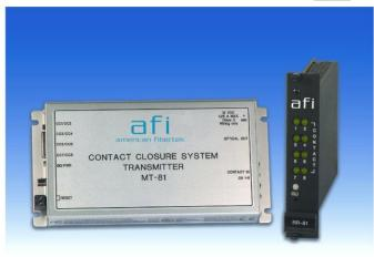
The American Fibertek 81-280 Series multiplexes 8 channels of dry non-latching contact closure on one multimode fiber. Both normally open and normally closed outputs are available. A set of 8 LEDs on the transmitter and the receiver units indicates the channel(s) status.
