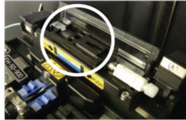
Figure 10: Holder used as heat shield
