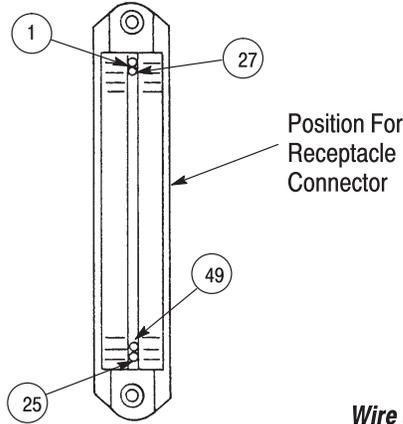
**Wire and Connector Placement for Terminating Receptacle Connector**
