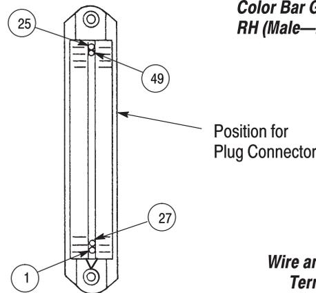
**Wire and Connector Placement for Terminating Plug Connector**
