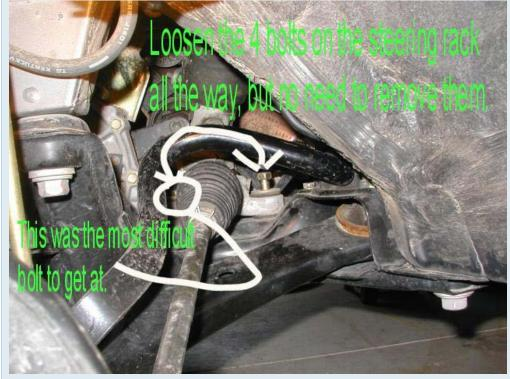
These two bolts on each side are very tight. An air impact wrench will be much safer to remove these bolts than a ratchet with a "cheater bar" because you could pull the car off of the jackstands. I have a wimpy air gun that wouldn't loosen one of them that I did carefully loosen with a ratchet. I loosened all 4, then removed the upper/more forward bolt on each side. These bolts are the only thing remaining holding up the cradle, so I loosened the rear bolts a ways, then
