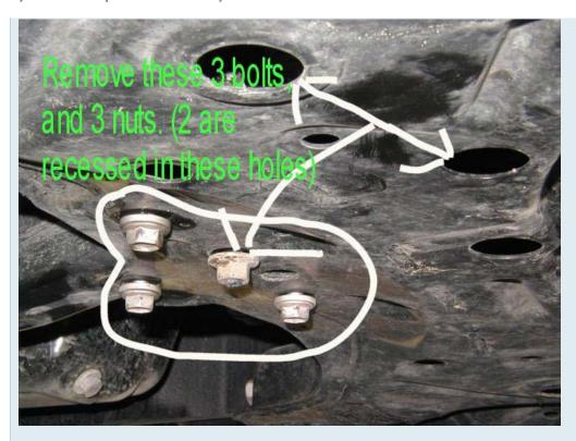
After the above bolts/nuts removed, place a floor jack under the center of the cradle. Bring jack up close to the cradle, but don't put any pressure on it, you're only going to use the jack to lower the cradle.
