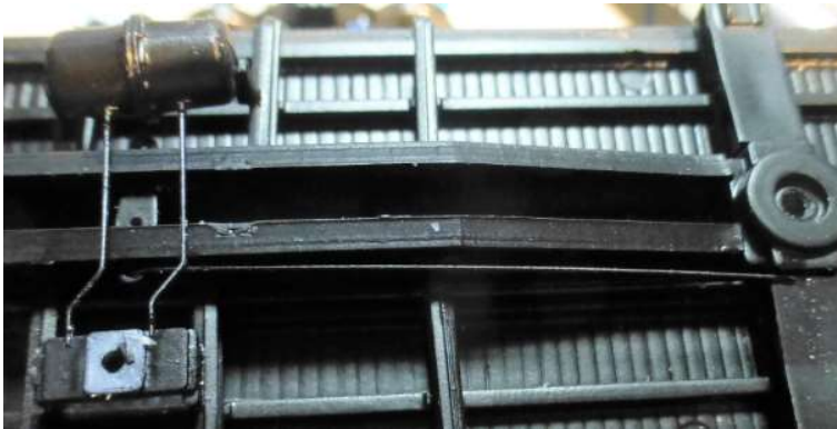
Shorten the long brake rod to fit between the dead lever and the A end bolster and glue in place.
