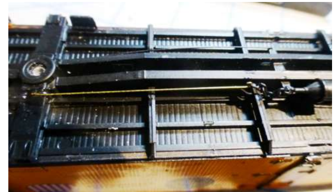
Trim the floating lever slightly and glue the cylinder to the center sill so that the open end of the clevis and chain line up with the end of the floating lever and glue there. The chain is too long to be realistic. Shorten it by about one half. Make new rod that will suspend the chain and extend to the brake fulcrum, or do in two pieces glued to the bolster.
