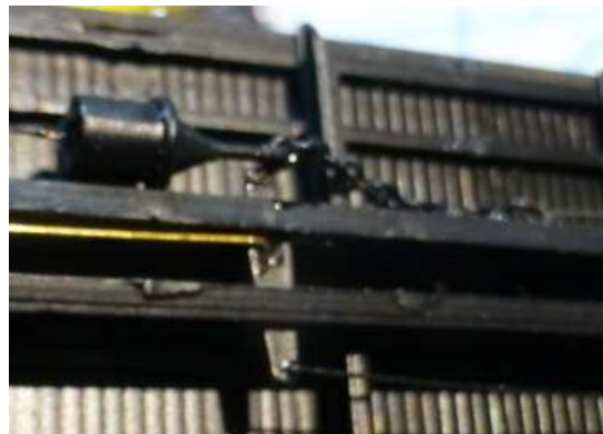
Trim the floating lever slightly and glue the cylinder to the center sill so that the open end of the clevis and chain line up with the end of the floating lever and glue there. The chain is too long to be realistic. Shorten it by about one half. Make new rod that will suspend the chain and extend to the brake fulcrum, or do in two pieces glued to the bolster.
