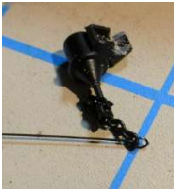
File a notch in the support bracket for the brake cylinder to fit over the train line. Drill a hole in the end of the cylinder for an air pipe. Note that the train line is mounted too close to the center sill, but to fix would involve redoing all of the needle beams.
