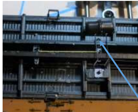
Make a connecting rod to fit between the floating lever and the dead lever of brass wire.
