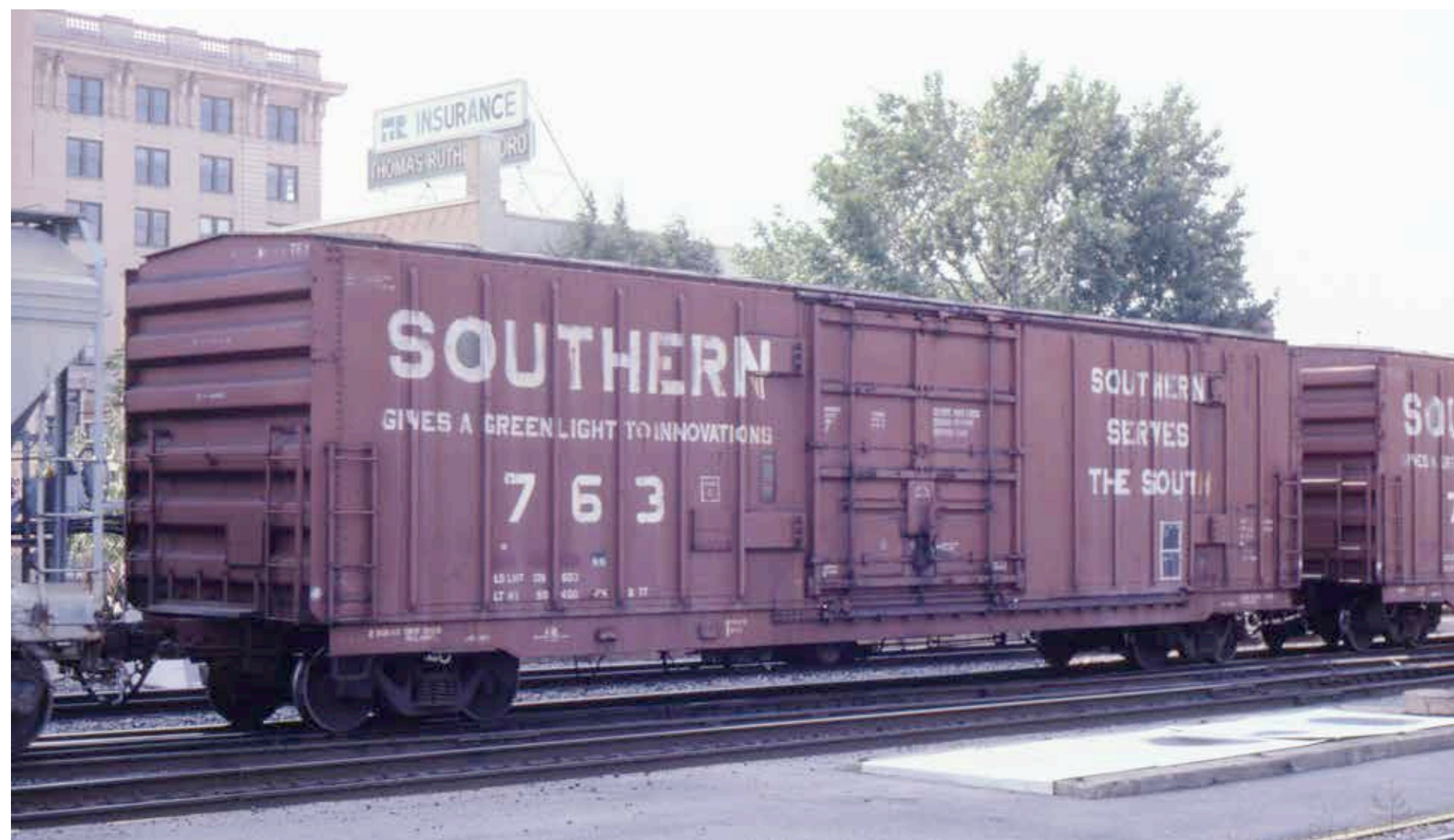
Southern 763 and NCP-177 cousin 795 are passing through Roanoke, VA on They are both from the first order of insulated box cars built by Fruit Growers for the Southern.
