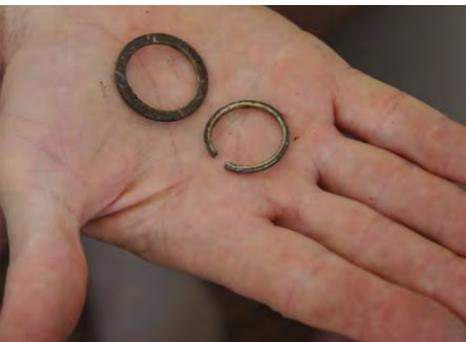
Circlip & washer. Retain for reassembly
