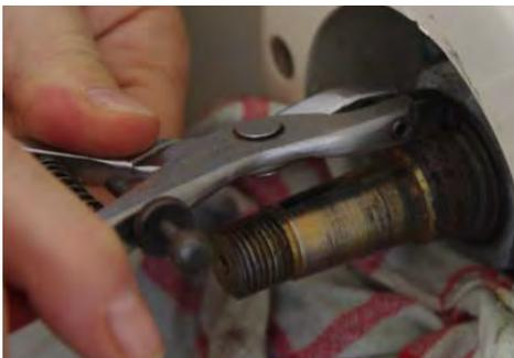
Remove the Circlip and washer with Circlip Pliers, or with needle nose pliers and/or a screwdriver.
