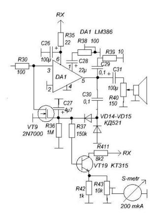
By resistor R42 we calibrate indications of S-meter, as which it is possible to apply the milliammeter with a current of arrow full deflexion up to 200-300mkA. At feeding of 50mkV on antenna input of the transceiver, the arrow of S-meter must show 9 points.
