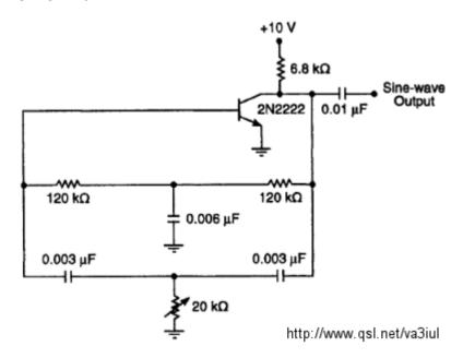
Here is the (VA3IUL) circuit I used for testing my BITX80v3 . It is injected directly into the mic input .
