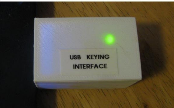
Completed optically isolated keying interface connected to PC's USB port. The SMD LED keying monitor is visible through a thinned out region of the 3D printed top cover.
