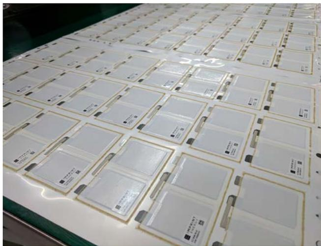
*Shown here: scores of Imprint Energy batteries, printed by a manufacturing partner using standard commercial equipment.*
